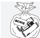
If the instrument is wet, it must be dried prior to storage.
